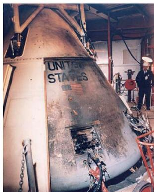
图2 阿波罗1号起火残骸(图片来源:<http://roll.sohu.com/20160322/n441477579.shtml>)
